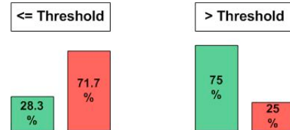
Figure 1: Distribution of non-defect-prone (green) and defect-prone (red) instances in case of a low and a high level of refactorings.
