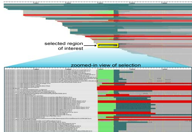
Figure 4: Identifying ArgoUML version changes between release VERSION_0_14_ALPHA_1 and release VERSION_0_14_F that contain the word “issue” in their commit comment. Inset shows a zoomed-in region, for better insight.
