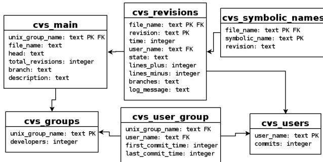
Figure 1: Entity-relation diagram of the CVS database.
